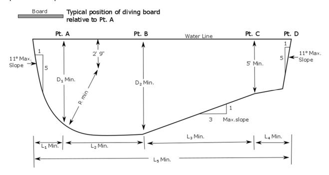
Note: L<sub>4</sub> is a minimum dimension to allow sufficient length opposite the board. This may of course be lengthened to form the shallow portion of the pool.
